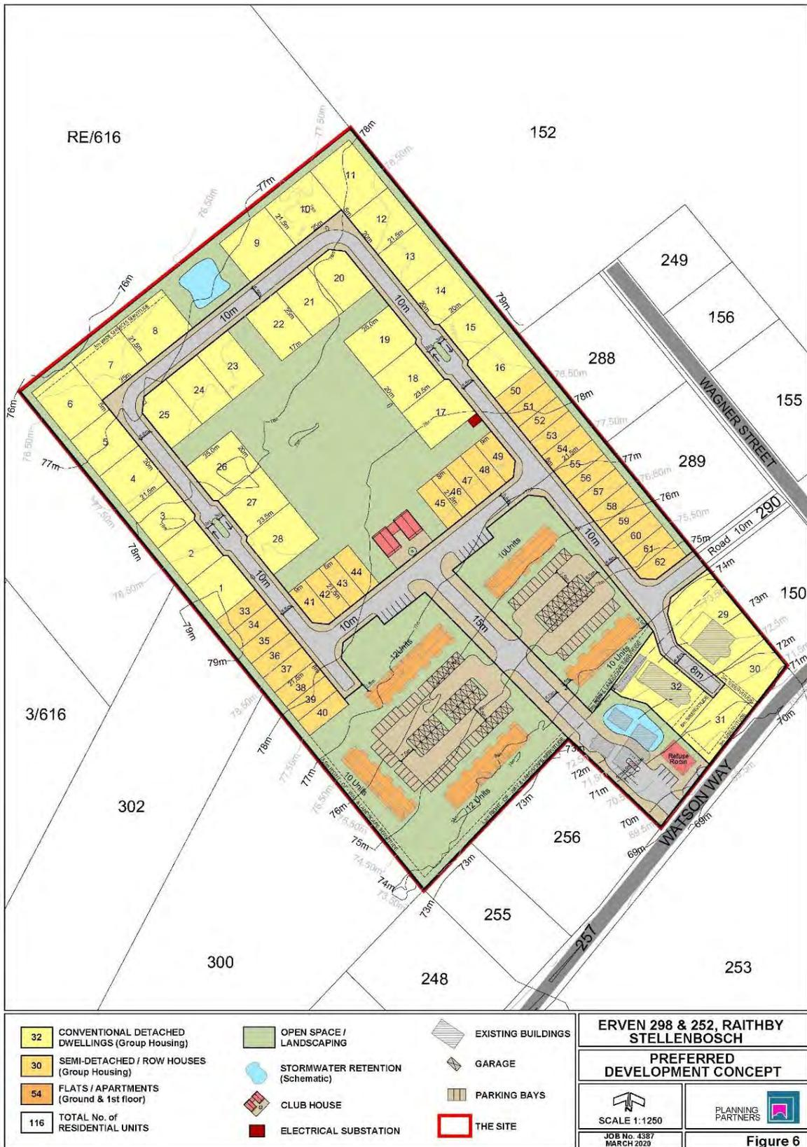
Figure A: Layout of the Preferred Alternative (Alternative 2).
